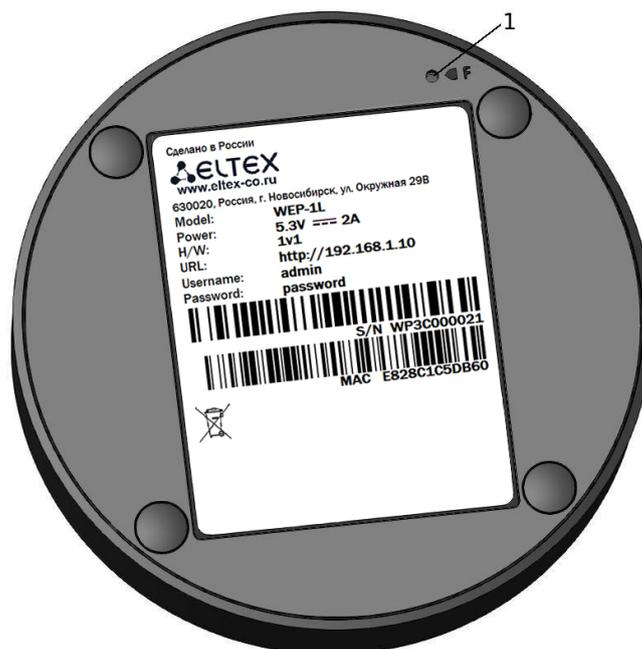
Figure 4 – Bottom panel of WEP-1L
