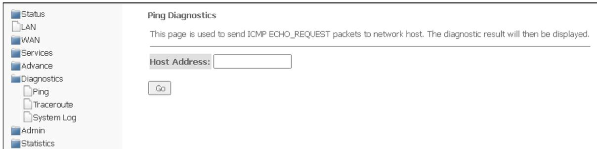
To check the availability of the connected device, enter its IP address in the **Host Address** field and click **Go**.
