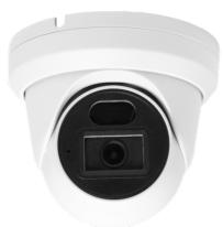
**SV-BA314-E** wired IP camera with a dome design provides a horizontal viewing angle of  $100^{\circ}$  and is equipped with a 4 MP CMOS matrix for clear video with a resolution of up to  $2560 \times 1440$ . The device has a night shooting mode (IR illumination), motion detection system and the function of saving the video archive to a memory card or network storage<sup>1</sup>. The camera is equipped with a RJ-45 connector with support for basic network protocols.
